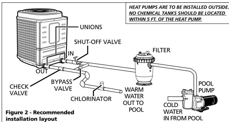
Figure 2 - Recommended installation layout
