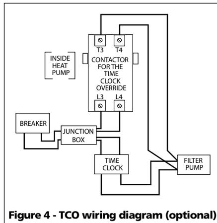
Figure 4 - TCO wiring diagram (optional)
